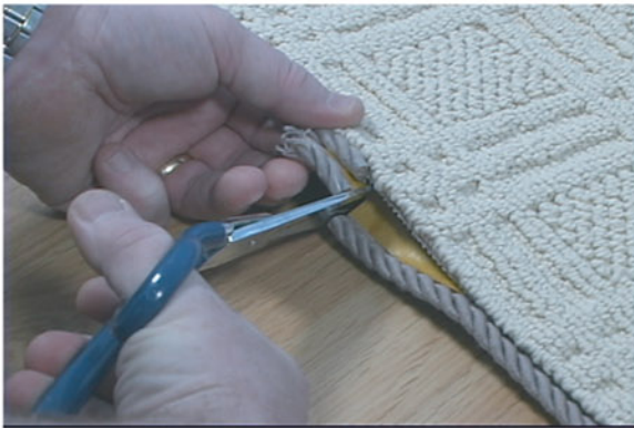
8) When joining the start and the end of the binding, apply Sellotape to the area where the cut will be made. This prevents the rope part of the binding from fraying when cut.
