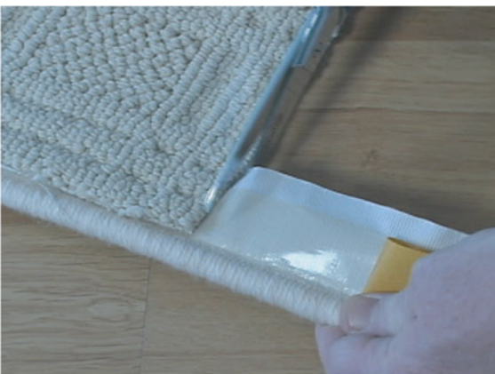
5) When going around a corner, cut the binding, not the rope! As shown above.
